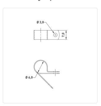
Bundle Diameter [mm]: 6 Color: Black Material: PA 6.6 Plastic Material Group: Mounting Hole [mm]: 3 Width [mm]:
