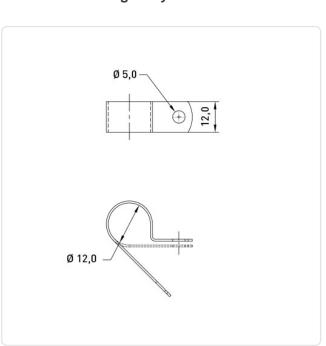
Bundle Diameter [mm]: 12 Color: Black Material: PA 6.6 Plastic Material Group: Mounting Hole [mm]: 5 Width [mm]: 12 Weight: 0.98g
