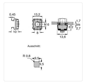
Finish: Galvanized Cage / Galvanized Nut
