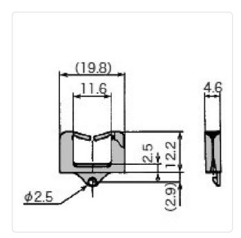
Color: Natural Height [mm]: 12.2 Material: PA 6.6 Material Group: Plastic Model: Screw-On
