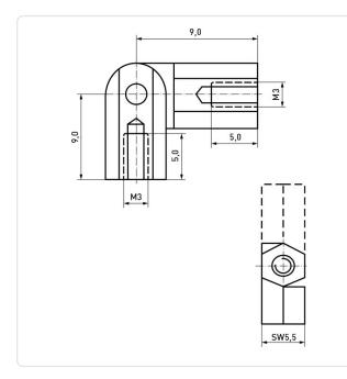
Finish: Nickel-Plated, 3 µm, E1E Leg Length 1 [mm]: 9 Leg Length 2 [mm]: 9 Length [mm]: 18 Material: Brass Material Group: Brass Model: Female/Female M3 Thread 1 Size: Thread 2 Size: М3 Weight: 3.09g Conformities: Reach RoHS SVHC
