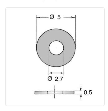
Color: Natural For Thread Size: M2.5 Height [mm]: 0.5 Inner Diameter [mm]: 2.7 Material: PA 6.0 Material Group: Plastic Outer Diameter [mm]: 5
