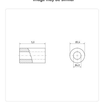
Finish: Plain For Thread Size: M2 Inner Diameter [mm]: 2.4 Length [mm]:
