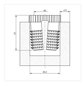
Finish: Plain Length [mm]: 4 Material: **Brass** Material Group: Brass Minimum Edge Distance [mm]: 2.0 Panel Hole Ø [mm]: 4 Thread Size: М3
