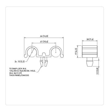
Bundle Diameter [mm]: 2,0-5,0 Color: Natural 16.8 Height [mm]: PA 6.6 Material: Material Group: **Plastic** Mounting Hole [mm]: 3.2 Width [mm]: 7.6 Weight: 0.27g
