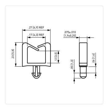
Bundle Diameter [mm]: 2,0-5,0 Color: Natural 5.8 Height [mm]: PA 6.6 Material: Material Group: **Plastic** Mounting Hole [mm]: 1.7 Panel Thickness [mm]: 1,6 mm Width [mm]: 6.9 Weight: 0.06g Conformities:
