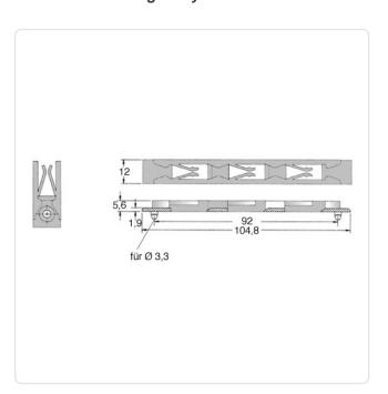
Color: Black Dist. Mounting Holes [mm]: 92.1 Flammability Class: UL94-V2 Length [mm]: 104.8
