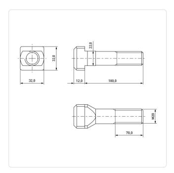
DIN/ISO: **DIN787** Plain Finish: Head Height [mm]: 12
