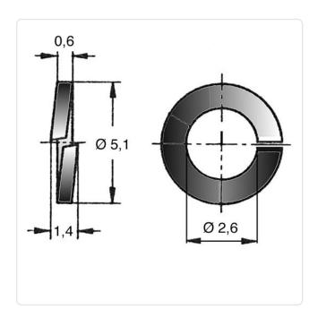
DIN/ISO: DIN127B Finish: Plain For Thread Size: M2.5 0.6 Height [mm]: Inner Diameter [mm]: 2.6
