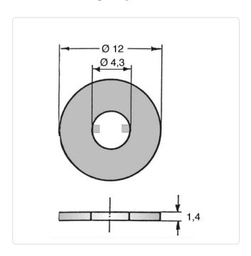
Color: Natural For Thread Size: M4 Height [mm]: 1.4 Inner Diameter [mm]: 4.3 Material: PA 6.0 Material Group: Plastic Outer Diameter [mm]: 12 Weight: 0.16g
