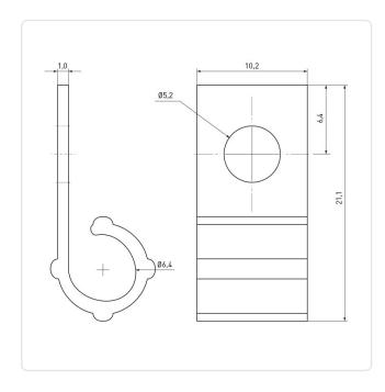
Bundle Diameter [mm]: 6,4 Color: Natural Flammability Class: UL94-V2 Length [mm]: 21.1 Material: PA 6.6 Material Group: **Plastic** Mounting Hole [mm]: 5.2 Thickness [mm]: 1 Width [mm]: 10.2 Weight: 0.55g
