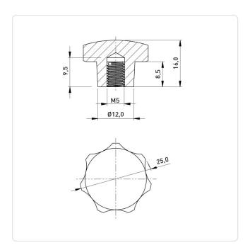
Color: Black Diameter [mm]: 25 Height [mm]: Material: Plastic Material Group: Plastic Thread Size: M4 Weight: 5.87g
