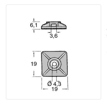
Cable Tie Width max. [mm]: 3.6 Color: Black Flammability Class: UL94-V2
