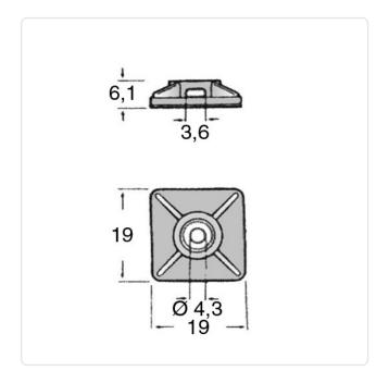
Cable Tie Width max. [mm]: 3.6 Color: Black Flammability Class: UL94-V2
