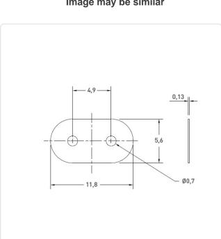
Flammability Class: UL94-V2 Length [mm]: 11.8 Material: Mylar Material Group: Plastic Mounting Hole [mm]: 0.7 Width [mm]: 5.6 Weight: 0.01g
