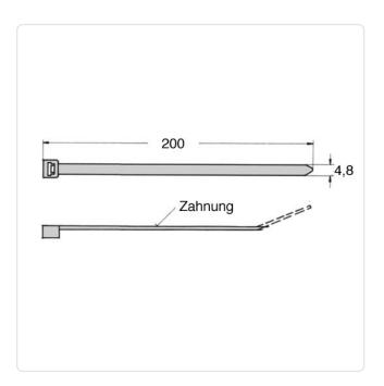
Bundle Diameter [mm]: 21,0-50,0 Color: Natural Flammability Class: UL94-V2 Length [mm]: 200 Material: PA 6.6 Material Group: **Plastic**
