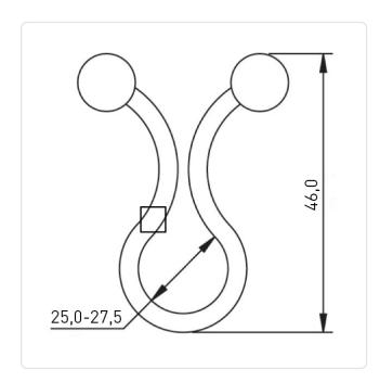
Bundle Diameter [mm]: 25,0-30,0 Color: Black Flammability Class: UL94-V2 Material: PA 6.6 Material Group: **Plastic** Weight: 0.91g
