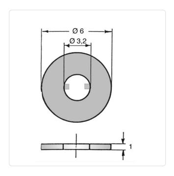
Color: Natural For Thread Size: МЗ Height [mm]: Inner Diameter [mm]: 3.2 Material: PA 6.0 Material Group: Plastic Outer Diameter [mm]: 6
