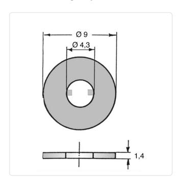
Color: Natural For Thread Size: M4 Height [mm]: 1.4 Inner Diameter [mm]: 4.3 Material: PA 6.0 Material Group: Plastic Outer Diameter [mm]: 9
