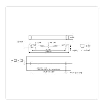
Bundle Diameter [mm]: 10,0-18,0 Color: White Height [mm]: 7.3 Material: PA 6.6 Material Group: **Plastic** Model: Flat Cable
