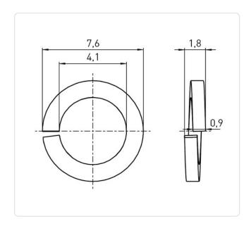
DIN/ISO: DIN127B Finish: Plain For Thread Size: M4 Height [mm]: 0.9 Inner Diameter [mm]: 4.1
