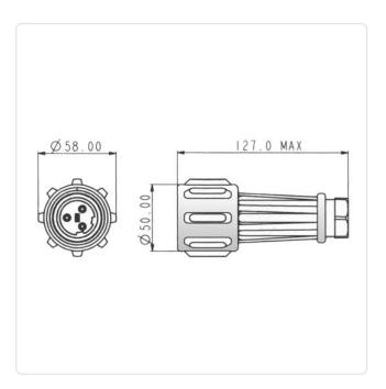
Amperage [A]: 32 Color: Black Protection Code: IP68 Weight: 134.5g
