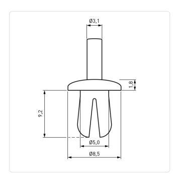
Color: Black UL94-V2 Flammability Class: Head Diameter [mm]: 8.5 Head Height [mm]: 1.8 Length [mm]: 9.2 Mandrel Diameter [mm]: 3.1 PA 6.6 Material: Material Group: Plastic
