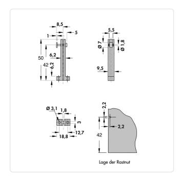
Color: Gray Dist. Mounting Holes [mm]: 12.7 Flammability Class: UL94-V0
