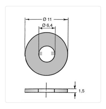
Color: Natural For Thread Size: M6 Height [mm]: 1.5 Inner Diameter [mm]: 6.4 Material: PA 6.0 Material Group: Plastic Outer Diameter [mm]: 11 Weight: 0.11g
