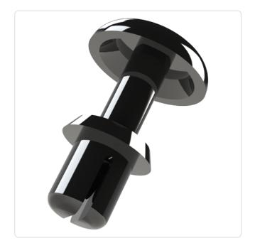
Color: Black UL94-V2 Flammability Class: Head Diameter [mm]: 6.4 Head Height [mm]: 1.6 Length [mm]: 4.5 Material: PA 6.6 Material Group: Plastic Model: removable Mounting Hole Range [mm]: Ø 3.1-3.2 2,0-3,0 Panel Thickness [mm]:
