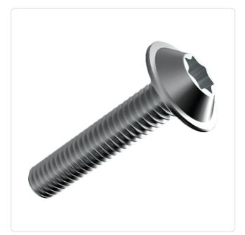
Actuator Size: Torx T10 DIN/ISO: ISO7380-2 Drive Type: **TORX** Plain Finish: Head Diameter [mm]: 6.9 Head Height [mm]: 1.65
