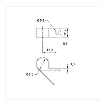
Bundle Diameter [mm]: 9,5 Color: Natural Distance Middle/Middle [mm]: 12.7 UL94-V2 Flammability Class: Material: PA 6.6 Material Group: Plastic Mounting Hole [mm]: 5.2 Thickness [mm]: 1.3 Width [mm]: 12.7
