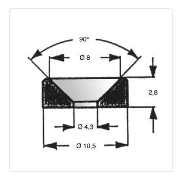
Color: White For Thread Size: M4 Height [mm]: 2.8 Inner Diameter [mm]: 4.3 Material: PA 6.0 Material Group: Plastic Outer Diameter [mm]: 10.5 Weight: 0.19g
