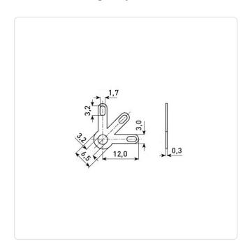
Finish: Plain Inner Diameter [mm]: 3.2 Length [mm]: 12 Material: **Brass** Material Group: **Brass** Outer Diameter [mm]: 6.5 Weight: 0.33g
