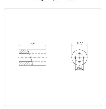
Finish: Plain For Thread Size: M6 Inner Diameter [mm]: 6.4 Length [mm]:
