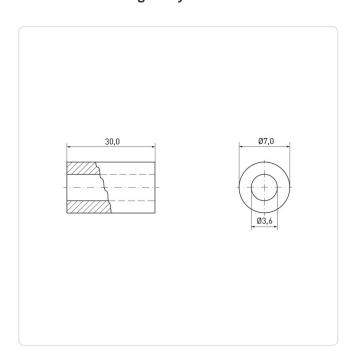
Color: Black Flammability Class: UL94-V0 For Thread Size: M3.5 Inner Diameter [mm]: 3.6 Length [mm]: 30
