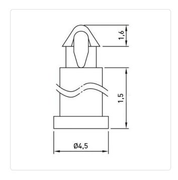
Color: Natural Flammability Class: UL94-V2 Length [mm]: 1.5 Material: PA 6.6 Material Group: **Plastic** Panel Hole Ø [mm]: 2.5
