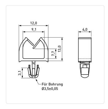
Bundle Diameter [mm]: 4,0-9,0 Color: Natural Height [mm]: 13 Material: PA 6.6 Material Group: **Plastic** Mounting Hole [mm]: 3.5 Panel Thickness [mm]: 1,6 mm Width [mm]: 12 Weight: 0.23g
