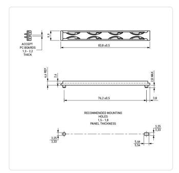
Color: Black Dist. Mounting Holes [mm]: 76.2 Flammability Class: UL94-V0 Length [mm]: 83.5
