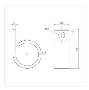
Bundle Diameter [mm]: 12,7 Color: Natural Flammability Class: UL94-V2 Length [mm]: 29.4 Material: PA 6.6 Material Group: **Plastic** Mounting Hole [mm]: 5.2 Thickness [mm]: 1.8 Width [mm]: 10.2 Weight: 1.41g
