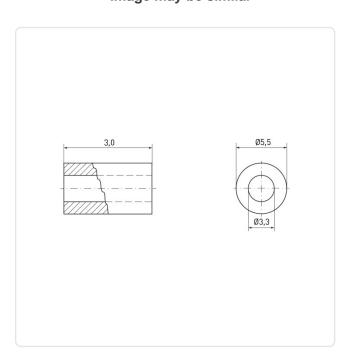
Finish: Plain For Thread Size: M3 Inner Diameter [mm]: 3.3 Length [mm]:
