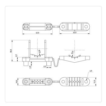
Cable diameter [mm]: Ø 10,8-18,5 Color: Natural Material: PA 6.6 Material Group: Plastic Max. Panel Thickness [mm]: 1.5 Panel Thickness Range [mm]: 20x20
