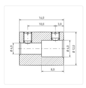
Height [mm]: 16 Inner Diameter [mm]: 6 Material: **Brass** Material Group: Brass
