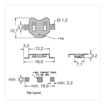
Battery Type: Cell Dia. 12mm
