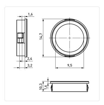
Color: Black Inner Diameter [mm]: 9.5 Material: PA 6.6 Material Group: Plastic Max. Panel Thickness [mm]: 3.2 Mounting Hole [mm]: 12.7 Weight: 0.54g
