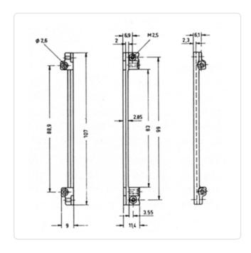
Color: Gray Dist. Mounting Holes [mm]: 88.9 Flammability Class: UL94-V0 Length [mm]: 107 Material: **Plastic** Plastic Material Group: Weight: 2.79g
