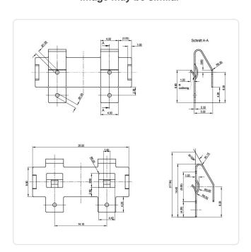
Battery Type: AA-Mignon Finish: Tin-Plated Material: Steel Material Group: Stahl Width [mm]: 14.3 Weight: 0.92g
