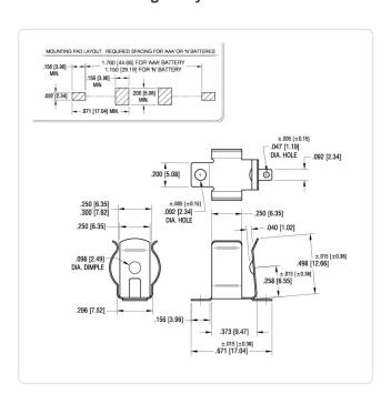
Battery Type: AAA-Micro Finish: Tin-Plated Material: Spring Steel
