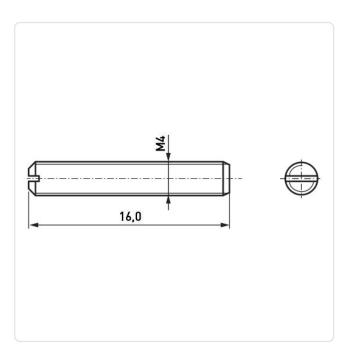
Color: Natural DIN/ISO: ISO4766 Drive Type: Slotted Flammability Class: UL94-V2 Length [mm]: 16 Material: PA 6.6 Material Group: Plastic Point Type: Flat Point Thread Size: M4
