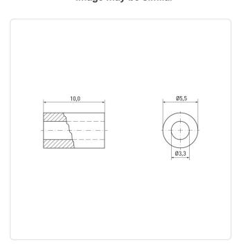
Finish: Plain For Thread Size: M3 Inner Diameter [mm]: 3.3 Length [mm]: 10
