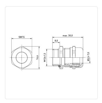
AF / OD [mm]: 15 Color: Black Material: PA 6.0 Material Group: Plastic Mounting Hole [mm]: 12.5 Panel Thickness Range [mm]: 3.5-7,0 Protection Code: **IP68** Thread Size: M12 Weight: 3.31g
